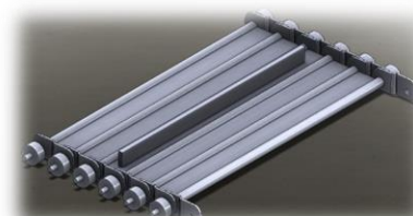
Slat/Hinged Type Belt Configuration
